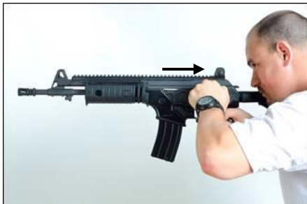
Figure 3-6: Cocking and Loading the Rifle
