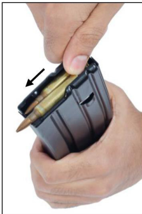
Figure 3-2: Unloading the Magazine
