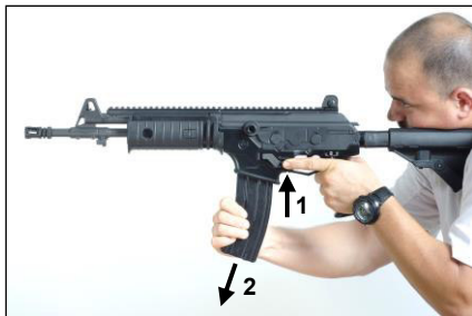
Figure 3-5: Removing the Magazine (2)
