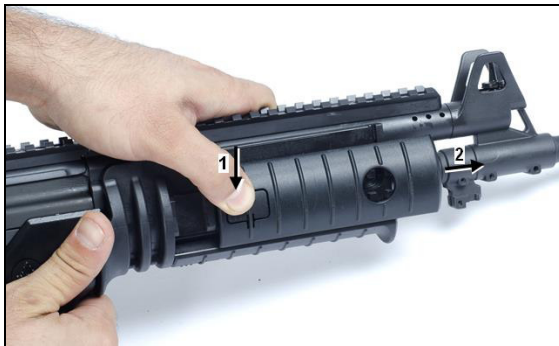
Figure 4-14: Removing the Rail Covers
