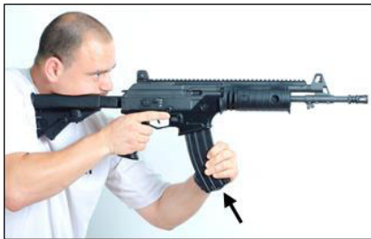
Figure 3-3: Inserting the Magazine
