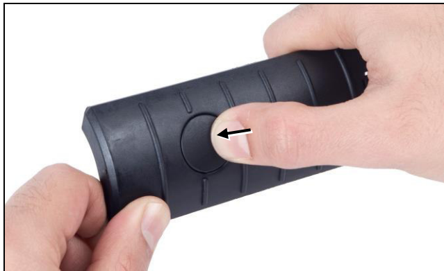
Figure 4-15: Removing the Button
