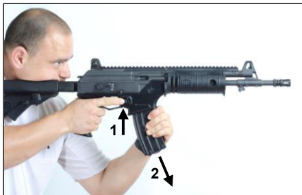
Figure 3-4: Removing the Magazine (1)
