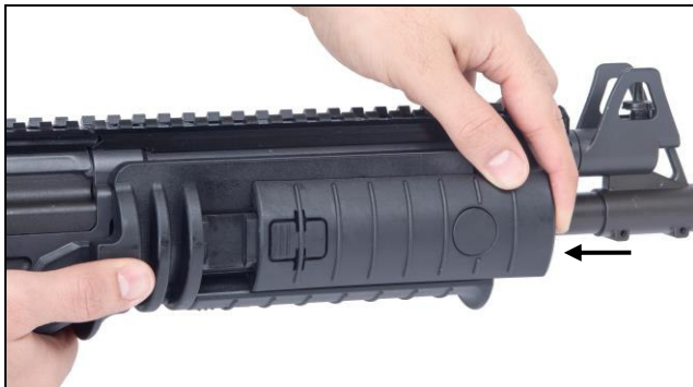
Figure 4-17: Inserting the Rail Covers
