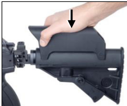
Figure 4-24: Installing the Cheek Rest
