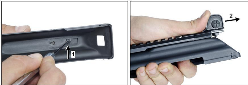
Figure 4-28: Removing the Rear Sight
