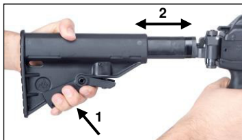
Figure 4-20: Buttstock Length Adjustment
